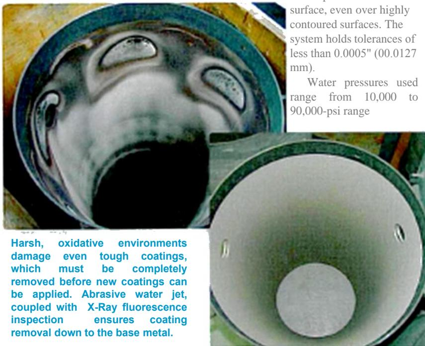
Harsh, oxidative environments damage even tough coatings, which must be completely removed before new coatings can be applied. Abrasive water jet, coupled with X-Ray fluorescence inspection ensures coating removal down to the base metal.
