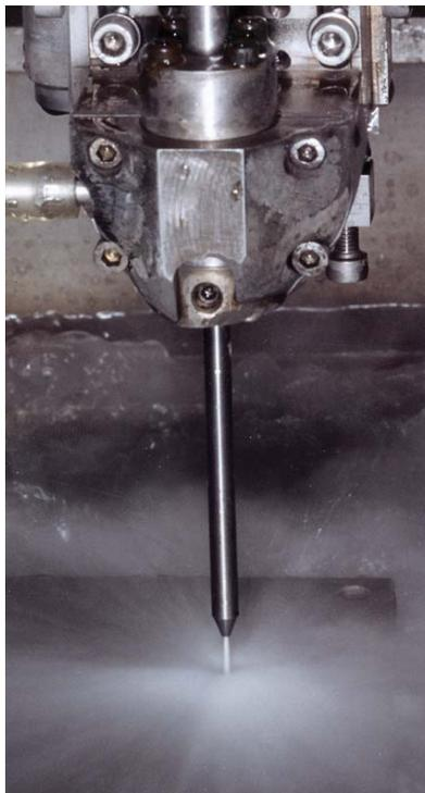
ing in iterative steps. Much like a machine tool, the material removal rates are controlled by speeds, feeds, pressures and material flow. Having increased control over the surface conditions offers a better TBC bond strength, which can result in a longer, more effective service life for each refurbished part.
