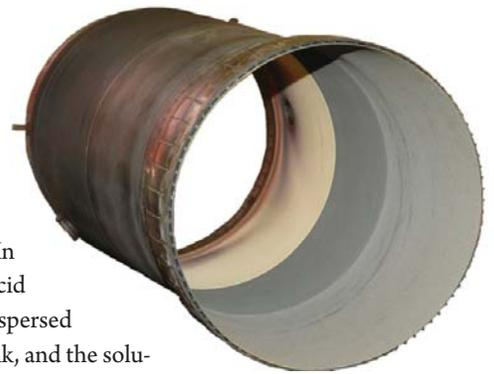
**Parts such as this industrial gas turbine liner are good candidates for the AWJ process because of their need for uniform coating removal during refurbishing.**
