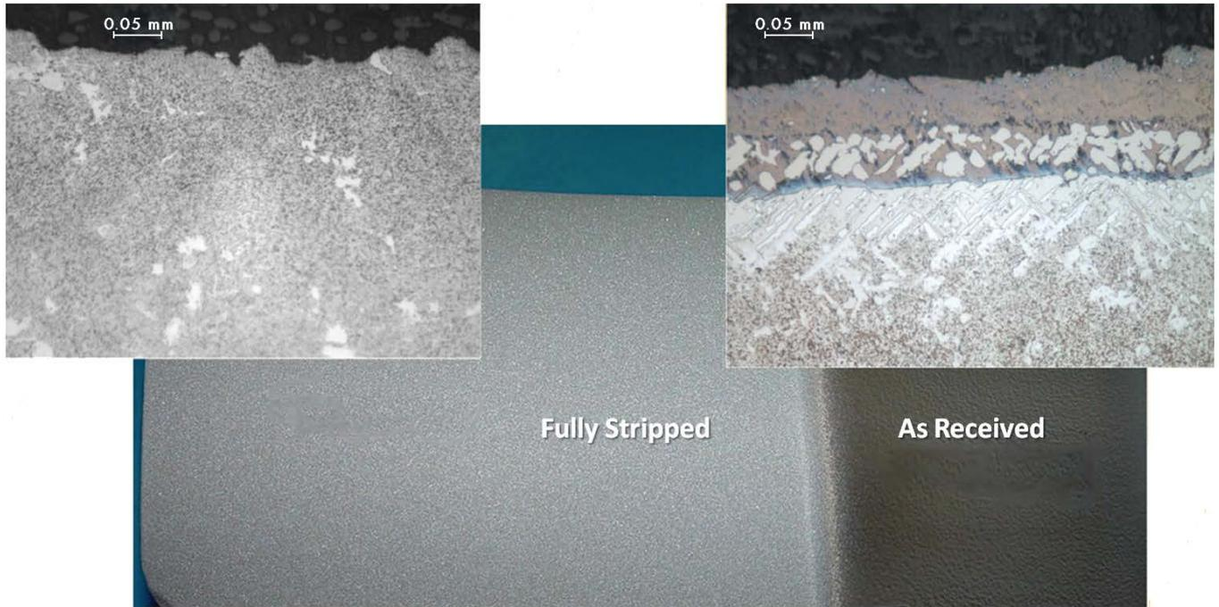
Coating removal - IGT Bucket: the photo above shows the as received condition on the right and the transition to a fully stripped coating on the left. The part was not masked and allowed for a smooth gradient from the coated to the stripped section.
